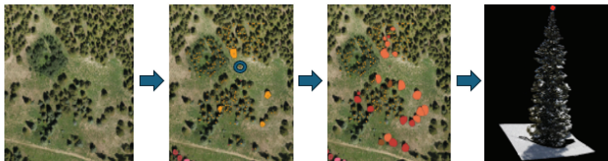
Figure 7: Workflow process Left-Right: Raw UAS imagery, point cloud generated tree tops + ground truth species ID, manual crown polygon clips according to species, final clipped tree.
