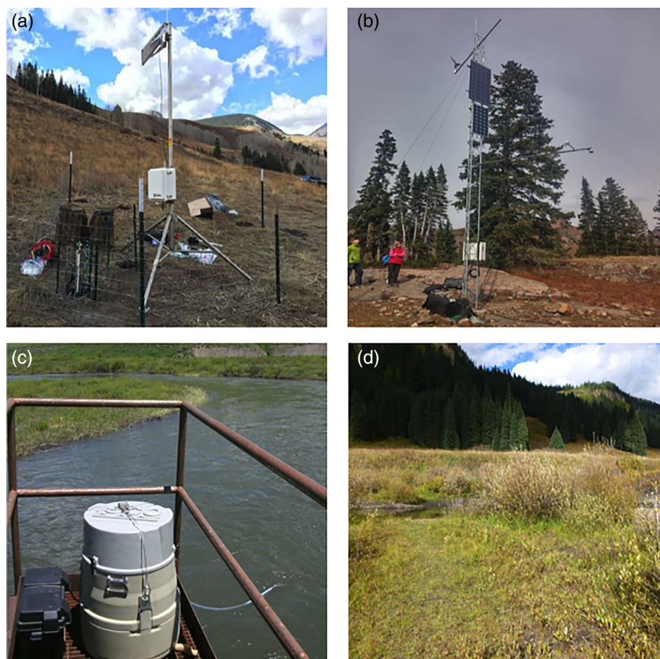
FIGURE 2 Photographs of some field locations and infrastructure installations in the ER: (a) hillslope borehole to measure subsurface water and carbon (b) weather station in the alpine zone (c) Pumphouse ISCO sampler for discharge and solute flux measurements (d) a plot to study impacts of early snowmelt on vegetation at a subalpine location along an elevation gradient
