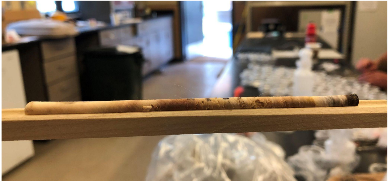
Figure 4: An aspen core sample after being glued into its wooden mount
