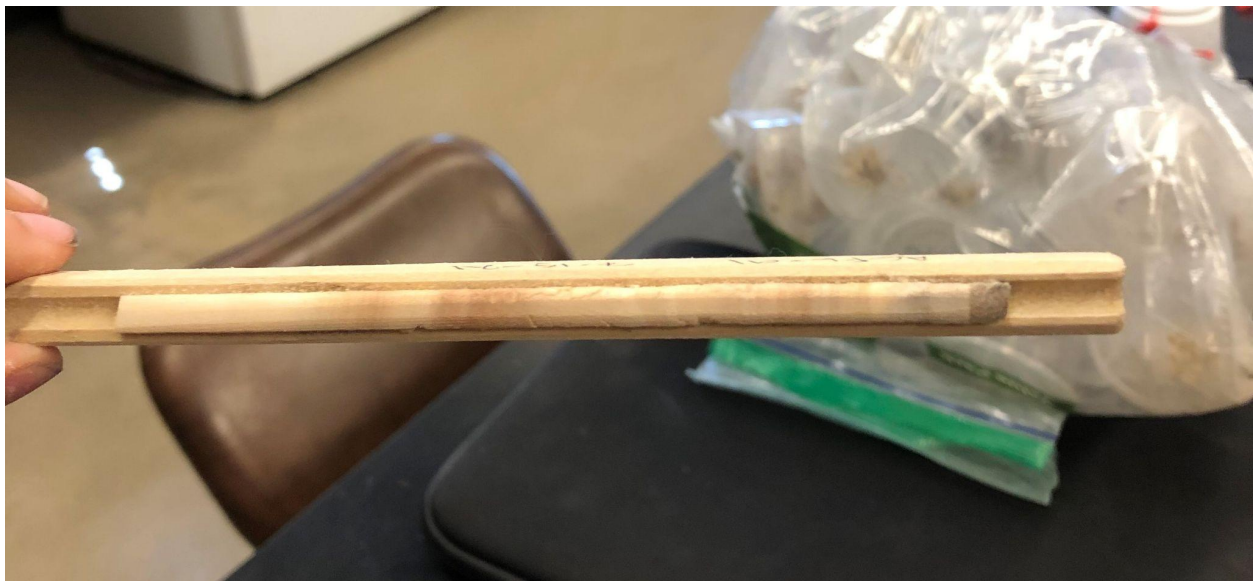
Figure 5: The same aspen core sample (Figure 1) after sanding using all four levels of grit paper.
