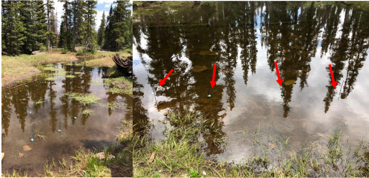
Figure 2: On the left, an image of a pond containing 24 NDS treatments. On the right, an image of one set of 4 NDS treatments, marked with red arrows.
