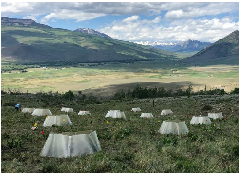
Figure 2. Low elevation site located near Almont, CO where open-top chambers are installed which warms air and soil temperature by \sim 2^{\circ}\text{C} .
