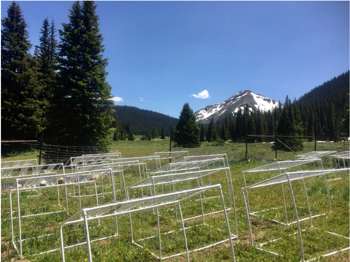
Figure J2. Deployment of rainout shelters in June 2017. Shelters were implemented in a checkerboard rather than randomized pattern due to space constraints in the garden.
