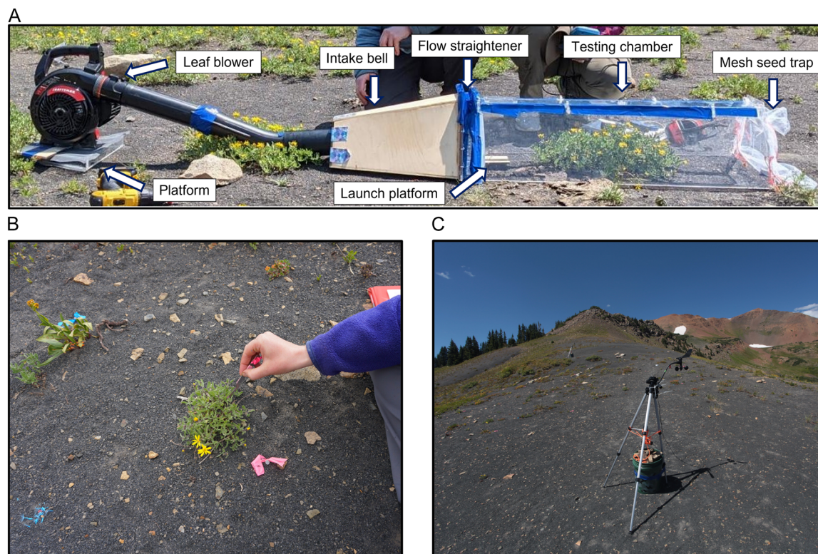
FIGURE 3 (A) Seed trapping setup. (B) The insertion of a seed into a Heterotheca villosa plant during the retention experiment. Blue-dyed seeds in the paired nonvegetated site are visible in the lower left corner. A second focal plant ( Senecio crassulus , marked with blue flagging) is visible in the background. (C) A cup anemometer in the retention experiment. A second cup anemometer is visible in the background.
