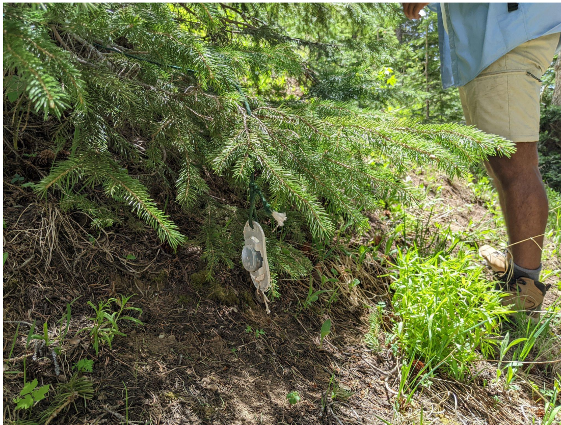
Figure 2. RG5 Sensor found unburied and approximately 5-8 cm above ground surface. Sensor still took temperature measurements.
